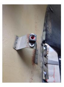
The snubber plate mounted to the O360 engine. Note the wear marks from a worn out snubber. A new snubber plate mounted to the forward nose of the cowling. Note: earlier C172 cowlings had landing light fixtures in lieu of the snubber bracket.
