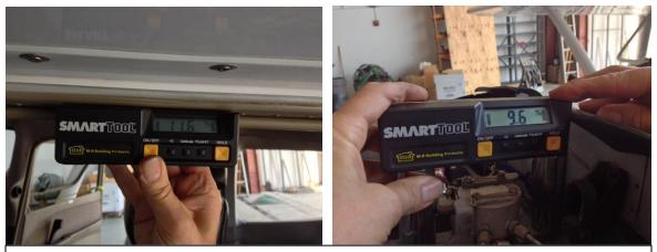
Airframe level (measured at door post) was 11.6 degrees nose up. The engine level was 9.6 nose up. This indicates that the engine is sagging or has an inclination of 2.0 degrees down.
