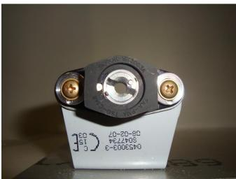
with the corresponding hole (centered), we have neutralized static stress. We can also "shift" the cowling in all axis to match paint lines, but most important, prevent the engine from hitting the cowling, particularly as a result of a firm landing. There are other factors, but the engine striking the cowling is the most notorious for failures.
