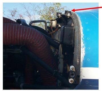
Here is another common observation. Mounts are angled excessively up or down. With the mount removed, the mounting bracket can be "aligned" to agree with the cowling slope by bending the 2-piece bracket, clamp, and re-drill the mounting holes. This may (probably will) relocate the mount center relative to the cowling hole. Using the SK2003-AW Camwashers. this mount is now faced (angled properly) with the cowling and centered to relieve static load.
