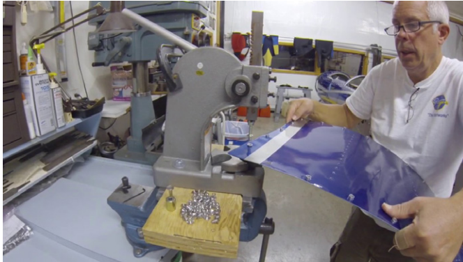
For production, use Skybolt® tool dies with common 2-ton Arbor Presses. For installation video, see www.skybolt.com/Instructions -or- https://youtu.be/2r0-D3k7UZs
