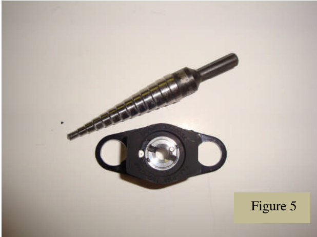
Drill mount holes to 7/16” with Unibit-1 drill
